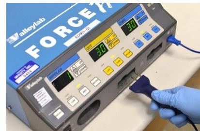
7. Based on the desired tissue effect the lowest energy settings should be used. It is not recommended to use CUT or COAG settings over 50 watts or any power setting and mode that results in an output voltage greater than 3000V. Consult the user manual of the electrosurgical unit (ESU) to determine the voltage output characteristics for different power settings and modes.
